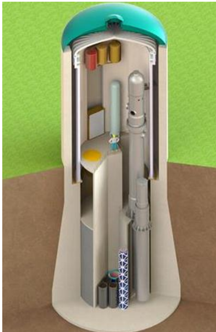
Containment structure and containment enclosure structure
