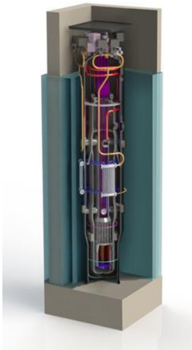
Reactor System Configuration of NuScale (Courtesy of NuScale Power Inc., with permission)
