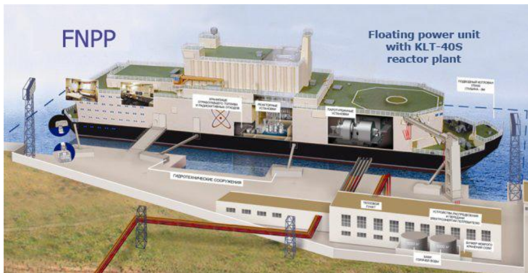
Possible floating power unit configuration (Courtesy of OKBM Afrikantov, with permission)
